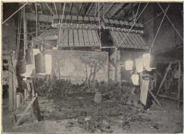
Fig. 6. Indoor Studio Setting for Outdoor Scene, Showing Lamp Arrangement for Artificial Lighting
